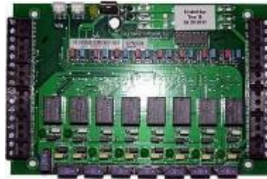
C8 lock control module
