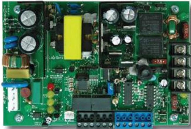
FPO Power Supply / Battery Charger
